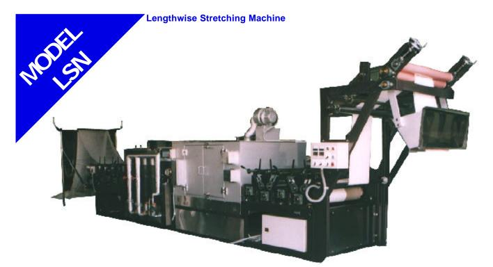
Netting produced by a netting machine requires a post treatment for better finish and increased knot fastness. The Model LSN series of lengthwise stretching machines allow you to produce netting that is ready for delivery. Due to the machines' high capacity and ease of use, it is possible to maintain a high production yield with minimum labor.
