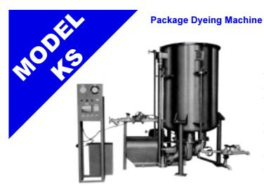
The Model KS package dyeing machine is designed and constructed for dyeing nets at high temperature under normal pressure. Nets are pressed tightly against a perforated carrier, and a dye solution is then circulated around and through the netting using a powerful hydraulic pump. This ensures deep, even penetration of dyestuff into all filaments and knots. The net knots are also fixed during the dyeing process.
