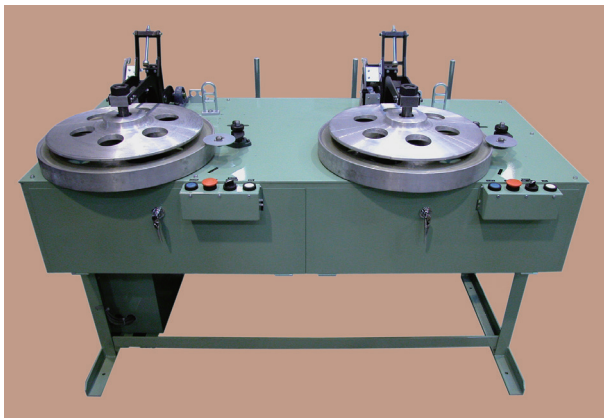
Model B-2E bobbin winder for Model GTA type 50-10.
